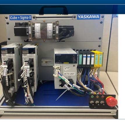
The iCube and Sigma-X multi-axis control portable demo unit serves as an excellent tool to demonstrate the features and benefits of both the iC9226M-FSoE and the Sigma-X series of SERVOPACKs and motors. The demo has been designed with a flexible architecture that allows for product demonstrations and application testing.
